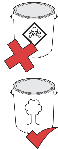
FIGURE 3: Substituting hazardous substances for less hazardous ones
